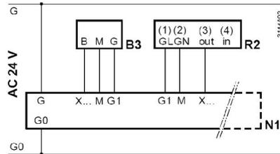
*Connection diagrams 3 and 4: Measuring section with CO<sub>2</sub>/VOC- and CO<sub>2</sub> evaluation.*
