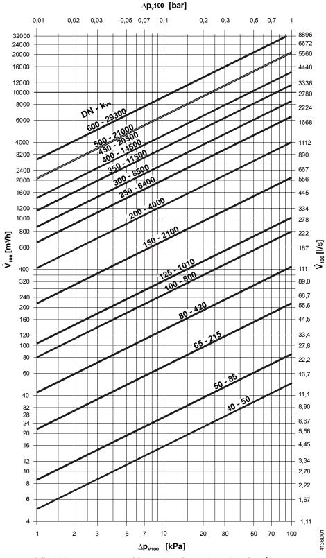
$\Delta p_{v100} \qquad \text{= Differential pressure across the fully open butterfly valve by a volume flow } \$_{100}$
