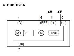
Tool = Configuration and maintenance interface (7-pin)
