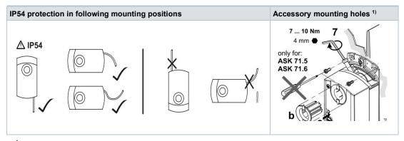
$oldsymbol{\Lambda}$  Not to be used for fixation of the actuator, use anti-rotation-bracket instead.
